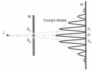
L is the light source. M stands for a "mask", which contains two slits,  $S_1$  and  $S_2$ . The light passes through the mask and gets projected onto a screen labeled N. The stripes on the figure indicate spots of varying intensity or brightness as shown below. The letters  $y_1$  and  $y_2$  indicate positions on the screen relative to the middle of the pattern (origin O).
