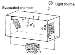
The  $\gamma$  symbols refer to "quantized oscillations of electromagnetic energy", which we (thankfully) now call *photons*, coming from the light source; the e<sup>-</sup> symbols refer to electrons which have left the electrode on the left and are attracted to the electrode on the right. The electrons can come off of the left electrode with varying amounts of energy.
