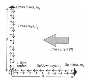
Using v to indicate the speed of the ether wind, we worked out in class the time for light to travel along the round-trip horizontal and vertical paths:
