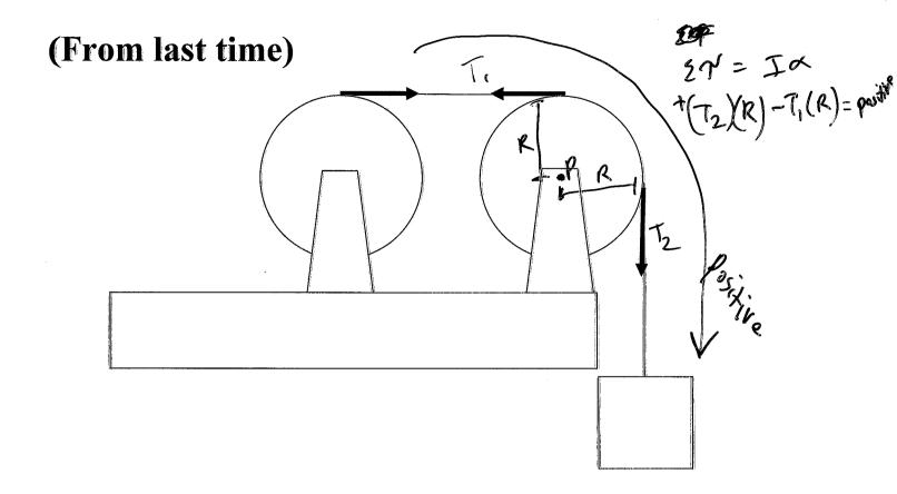
The left disk has a rope wrapped around its edge and the rope passes over a second disk. The two disks are identical and their **mass is significant**. As the system accelerates there is no slipping of the rope on either wheel and both wheels accelerate the same. The tension in the rope is
