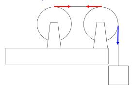
The left disk has a rope wrapped around its edge and the rope passes over a second disk. The two disks are identical and their **mass is significant**. As the system accelerates there is no slipping of the rope on either wheel and both wheels accelerate the same. The tension in the rope is
