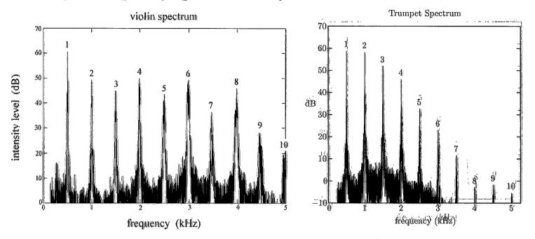
Note: the measured waves are combinations of sine waves. All of the frequencies present are multiples of the 1<sup>st</sup> harmonic (the pitch you hear)
