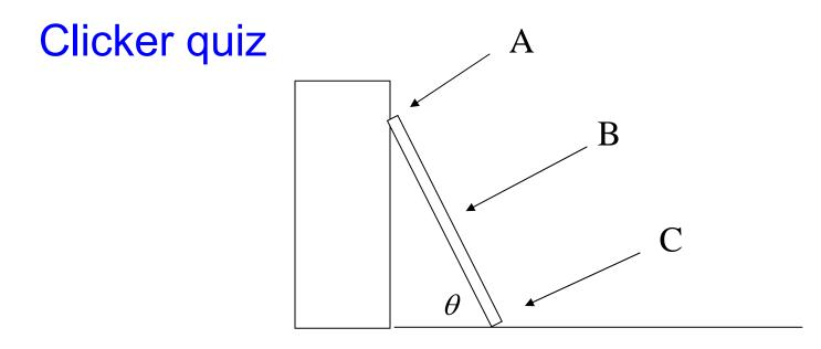
To solve the problem, we need to use  $\Sigma \tau = 0...$  but about which "pivot point" should we compute the torques?
