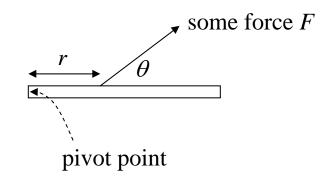
Positive/negative: Produces a **clockwise** rotation = **negative** Produces a **counter-clockwise** rotation = **positive**
