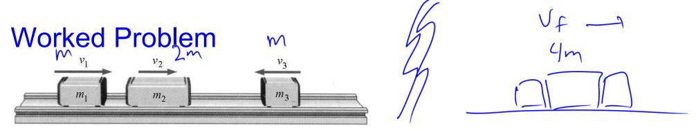
Three carts collide on an air track. Carts  $m_1$  and  $m_3$  have the same mass, and  $m_2$  has twice the mass. The initial velocities are 1.5 m/s, 1 m/s, and -1 m/s. The three stick together. What is the combined velocity after the collision? (magnitude and direction)
