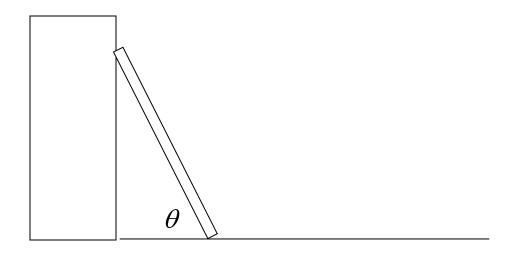
If  $\mu = 0.5 \rightarrow \theta = 36.9^{\circ}; \quad \mu = 0.7 \rightarrow \theta = 20.0^{\circ}; \quad \mu = 0.9 \rightarrow \theta = 6.0^{\circ}$ Answer:  $\theta = \tan^{-1}(1/(2\mu) - \mu/2)$
