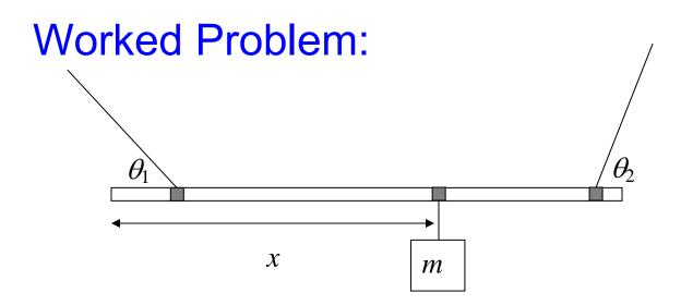
A 0.4 kg meterstick is suspended from pulleys and support pillars (not shown) via two strings at  $\theta_1 = 41.4^\circ$  and  $\theta_2 = 60^\circ$ , with tensions of 2 N and 3 N, respectively. The strings are attached at 10 cm and 5 cm from the two ends of the meterstick. The stick is *not* in equilibrium until an additional mass is hung from a point in the middle. Find the unknown *x* and *m*.
