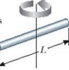
Long thin rod with rotation axis through end
