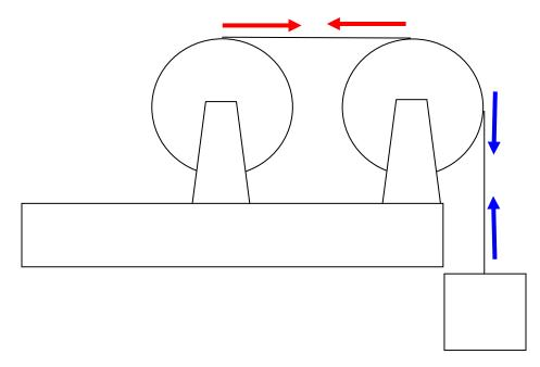
The left disk has a rope wrapped around its edge and the rope passes over a second disk. The two disks are identical and their **mass is significant**. As the system accelerates there is no slipping of the rope on either wheel; both wheels accelerate at the same rate. The tension in the rope is
