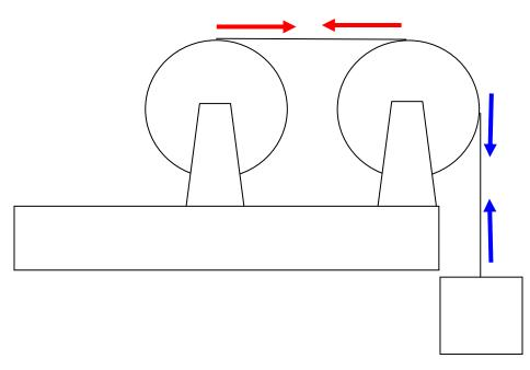
The left disk has a rope wrapped around its edge and the rope passes over a second disk. The two disks are identical and their **mass is significant**. As the system accelerates there is no slipping of the rope on either wheel; both wheels accelerate at the same rate. The tension in the rope is
