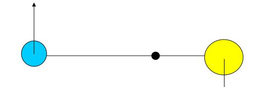
Two space stations are connected by a cable. They are rotating about their center of mass. Someone in the blue station pulls the cable in so they are each closer to the center of rotation. What happens?
