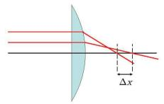
Hint: Here's a sketch for one of the rays, with the lens's radius of curvature expanded to a full circle, which should help you think about how to calculate the right distances.
