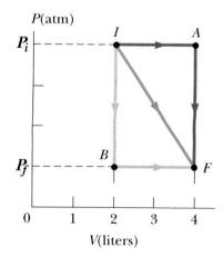
8-3. A monatomic ideal gas undergoes the thermodynamic process shown in the PV diagram in the figure.
