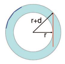
Hint: If the fiber/cladding combo (gray-blue, diameter d) were wrapped around a white cylinder of radius r, it would look something like the figure shown. The blue reflections on the upper-left would have no problem doing TIR. The red line on the right, however, represents a worst-case scenario that might run into trouble because of its steeper angle. (Answer: 15.0  $\mu$ m.)
