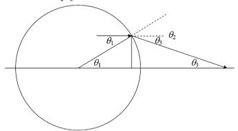
Final note: If you were to reverse the lens, so that the rays strike the curved side first, you would find  $\Delta x$  to be smaller. That gives rise to the first half of this optics rule about positioning these common "plano-convex" lenses: "Parallel rays to curved, diverging rays to flat."
