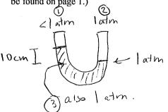
For the water in the left-hand section to end up 10 cm nigher than the water in the right-hand section. (Densities of air and water can be found on page 1.)
