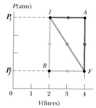
8-3. A monatomic ideal gas undergoes the thermodynamic process shown in the PV diagram in the figure. Determine whether each of the values (a)  $\Delta U$ , (b) Q, (c) W for the gas is positive, negative, or zero. (Note that W is the work done on the gas.)
