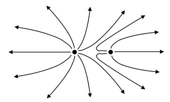
Notice that near each charge, the lines just go straight out from the circles; far away from both charges, the lines just go straight out from the center of the charges. And notice that the lines are most closely spaced near the charges, where the field is strongest—except for one point in between the two charges where the fields cancel each other out.
