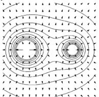
Notice how the arrows always point perpendicularly to the contours!
