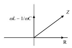
Step 2: Put in polar form,  $|Z_{eq}| \angle \phi$ :
