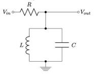
In this case I've written the equations in terms of the special frequency  $\omega_0 = \frac{1}{\sqrt{LC}}$ . You'll see the term  $Z_L//Z_C$  show up. It's left as an exercise for the reader (easily done with Mathematica) to show that that  $Z_L//Z_C = \frac{i\omega L}{1-\omega^2 LC} = \frac{i\omega L}{1-\omega^2/\omega_0^2}$ .
