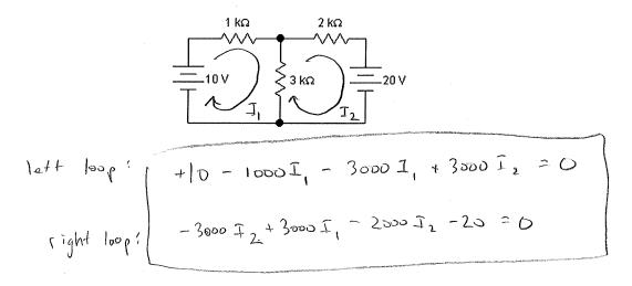
(b) Supposing you solve for  $I_1$  and  $I_2$  (you don't have to do this), how would you determine the voltage of the 3 k $\Omega$  resistor? Assume the top of the resistor is at a higher voltage than the bottom.
