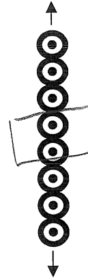
iii. infinite plane of wires with current I coming out of the page.
