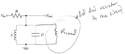
and add *another* resistor, let's call it  $R_{load}$ , going from  $V_{out}$  to ground. That represents the input impedance of the load circuit, i.e. whatever circuit you are hooking the filter up to. Notice that  $R_{load}$  is in parallel with L and C.
