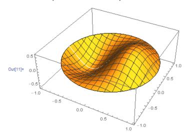
This is  $Ez = J_1\left(\frac{u_{11}s}{R}\right)\cos\phi$ . It's the first mode with  $\phi$  dependence. I used the "Arg" function as a trick to get  $\phi$ . Often we say  $\phi = \tan^{-1}\left(\frac{y}{x}\right)$ , but the  $\tan^{-1}$  function has problems in the  $2^{\rm nd}$  and  $3^{\rm rd}$  quadrants. Arg (the polar angle of a complex number) doesn't suffer from those issues.
