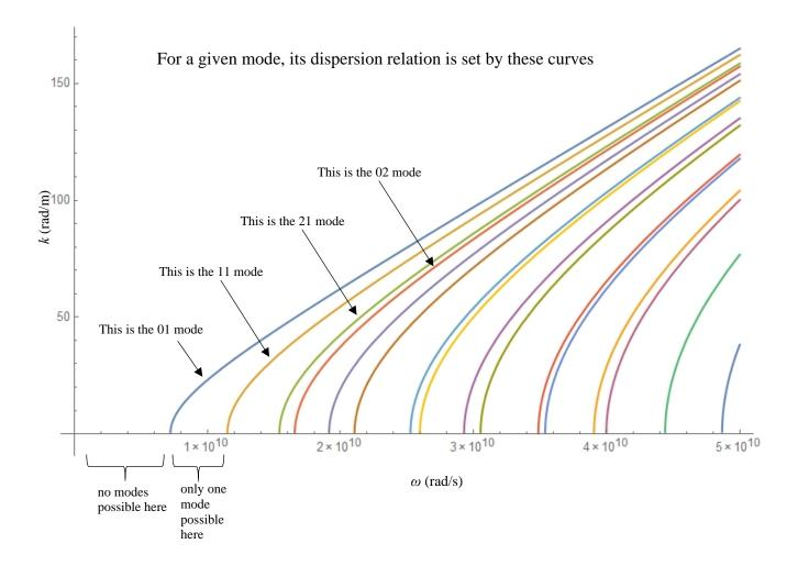
Note that these are the FIRST 16 modes, in the sense that  $\alpha$  goes from 0 to 3 and n goes from 1 to 4, but they are not necessarily the LOWEST 16 modes. For example, the ( $\alpha=4, n=1$ ) mode is lower than many of these that are shown (with its  $\omega_{cutoff}=2.28\times 10^{10}$  rad/s).
