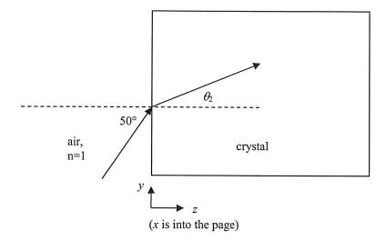
(a) If the light is s-polarized (i.e. electric field is in the x-direction), what is  $\theta_2$ ?
