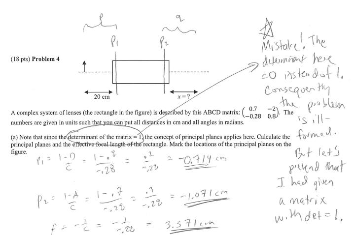
(b) An object is placed 20 cm to the left of the system, as shown by the vertical arrow. Use the principal planes along with the thin lens equation to determine where the image is formed relative to the end of the optical system, i.e. the distance marked x in the figure.
