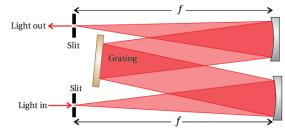
(a) What is the wavelength resolution (in nm) for light that is around  $\lambda = 500$  nm? I.e. about how far apart in  $\lambda$  will it be able to tell the difference between two very close wavelengths?
