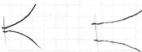
Note: Run light backwards in time, get focusing (and then diverging beam after it focuses to  $w_0$ )
