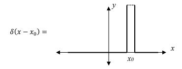
Shifting the position of the peak doesn't affect the total area if the integral is taken from  $-\infty$  to  $+\infty$ , or if the interval from *a* to *b* contains the peak.
