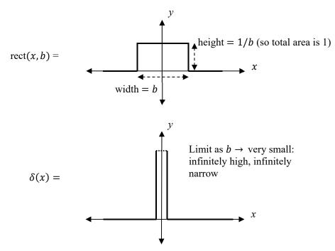
Note that the integral of the delta function is the area under the curve, and has been held constant at 1 throughout the limit process.
