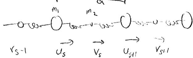
$$m_1 \frac{d^2 u_s}{dt^2} = c \left\{ (v_s - u_s) - (u_s - v_{s-1}) \right\}$$
