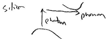
optical absorption at  $E_g$  less likely because need to absorb a photon as well (Si can't emit light easily also, for same reason) but GaAs = great!
