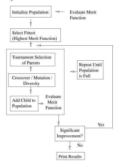
Figure 3: Schematic of the Genetic Algorithm
