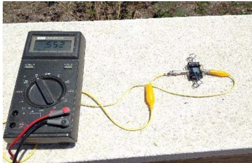
Ferritin-Mn open circuit voltage measurement
